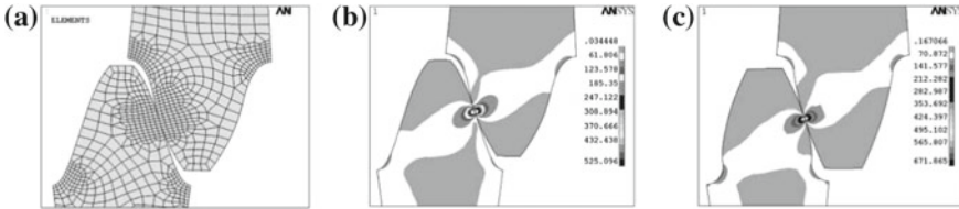
Fig. 4 a FEM Model b Stress distribution of cosine &c Involute profile [12]
