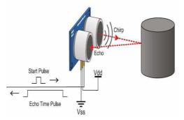
Fig. 4: Ultrasonic Sensor
