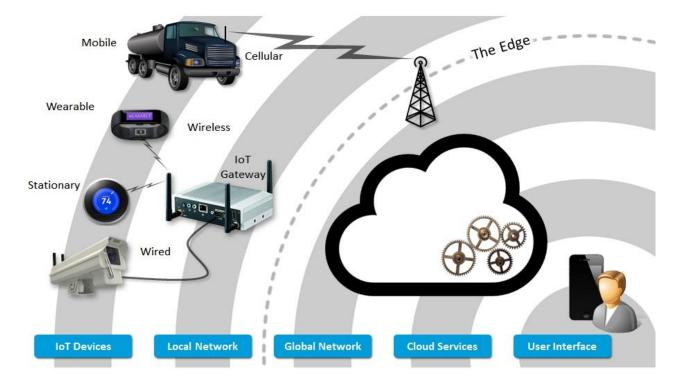
The architecture of FC accomplishes three basic layers, i.e., Cloud services layer in the top, Internet infrastructure layer in the middle, and Fog layer in the bottom level.
