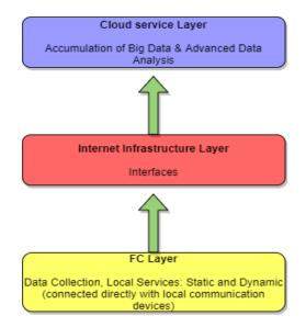
The data send by the communication devices like sensors, mobile devices, etc. are received by the Fog Node in the network of systems. The collected data from different sources may vary in their format. It requires data formatting to get all data in certain standard format. The Fog Node itself is installed with the applications to provide static services as well as dynamic services which will provide the output data to act according to the environmental changes.
