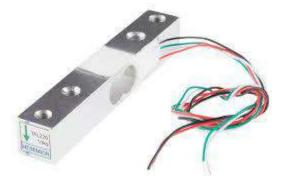
A **load cell** is a transducer which converts force into a measurable electrical output. Although there are many varieties of load cells, strain gage based load cells are the most commonly used.
