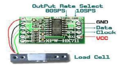
This Load Cell Amplifier is a small breakout board for the HX711 IC that allows you to easily read load cells to measure weight. By connecting the amplifier to your microcontroller you will be able to read the changes in the resistance of the load cell and with some calibration you'll be able to get very accurate weight measurements. This can be handy for creating your own industrial scale, process control, or simple presence detection.
