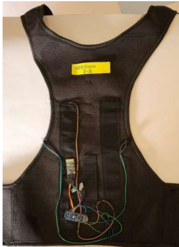
Figure 14: Posture Correction Device Version 2.2
